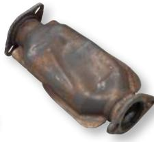
Impact under vehicle crushing converter
